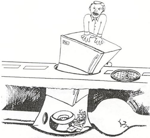
Normally, if a stoppage occurs in your neighborhood's main wastewater line, only the lowest level drains and toilets will be affected. A common point is floor drains located in basement areas.
