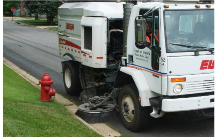
Brian Reynolds operates a regenerative air sweeper on the streets of Vienna. The vehicle blows hurricane force air down on one side and vacuums on the other side to create a turbulent suction which not only collects what the brush dislodges but also fine dust and particles. The technology is environmentally friendly and superior to the previous generation of sweeper which used a conveyor belt to carry the debris into a hopper.
